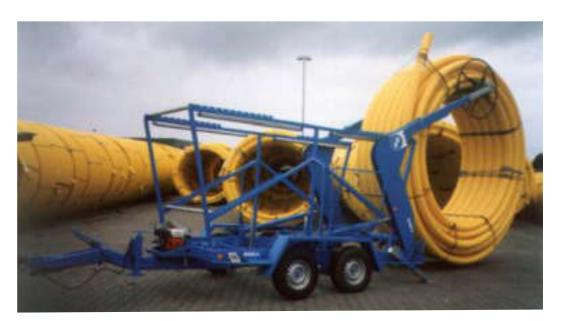
The BRT 20 is able to pick up, load and uncoil pipe coils without any help. Even laying coils can be picked up without any auxiliary equipment. Tube coils of varying diameters may be picked up with the aid of the vertical hydraulic jacks and put down on the bearing rollers. Then three guiding rollers are inserted on the inside of the coil, and the coil is ready for unreeling.
