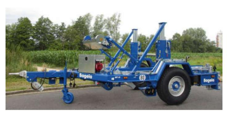
For winding and transportation of compact inline pipe of 400 mm dia., reels of an outer diameter of 3700 mm are needed. For carrying such large reels we have designed our trailer BRT 65 with an open rear side to enable the reel to be placed inside the trailer frame for being picked up. Serially the trailer is equipped with a rear gate to be opened to one side.
