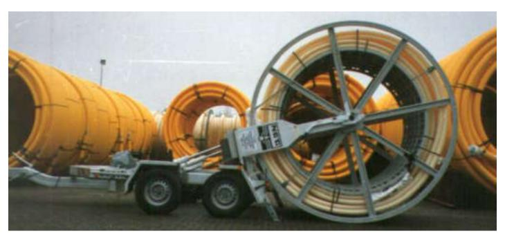
BRT 25 picking -up a U-liner drum
