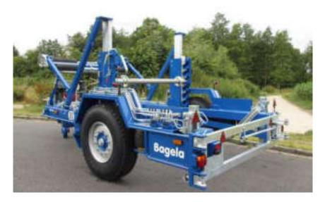
Two vertical pocket jacks, which may independently be moved up and down by an engine-driven hydraulic drive system and which are secured for transport by locking pins, lift the reel.
