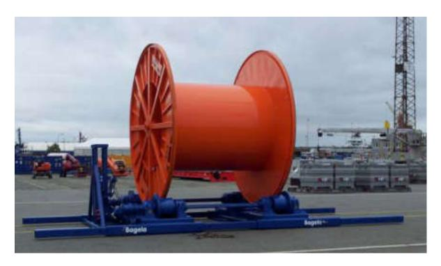
The KSP 80 pulls cable rests from a submarine cable ship and rewinds it directly on cable drums of up to 80,000 kg total weight. The drums get tensed up by the drive rollers. A tensile and braking force of up to 110 kN depending on the drum diameter.
