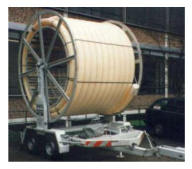
It is essential that contractors should adapt their tools and equipment to the development of underground tube renewal techniques. While tube manufacturers first and foremost think of the most efficient way of manufacturing and packing, tube laying contractors are faced with the problem of how to transport and install the tubing.
