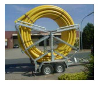
For BKT 18 up to BKT 27 • Uncoiling cage for special length 290 m, pipe dia.: 160 mm
