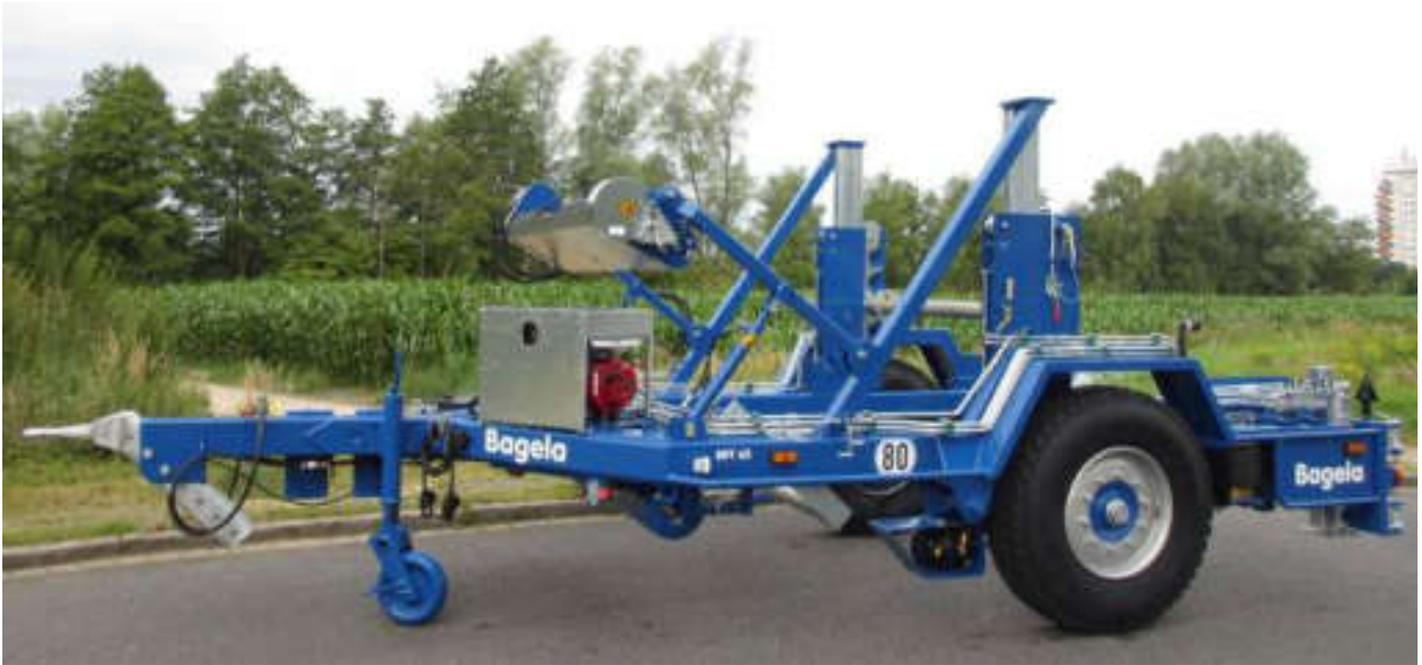
For winding and transportation of compact inline pipe of 400 mm dia., reels of an outer diameter of 3700 mm are needed. For carrying such large reels we have designed our trailer BRT 65 with an open rear side to enable the reel to be placed inside the trailer frame for being picked up. Serially the trailer is equipped with a rear gate to be opened to one side.
