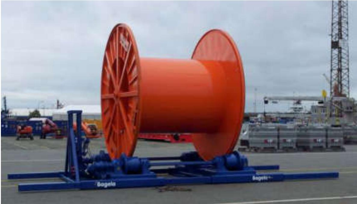
The KSP 80 pulls cable rests from a submarine cable ship and rewinds it directly on cable drums of up to 80,000 kg total weight. The drums get tensed up by the drive rollers. A tensile and braking force of up to 110 kN depending on the drum diameter.
