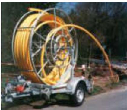
The Coil Reels type RH 40 and RH 63 may be used in a cable drum trailer, without the rack.
