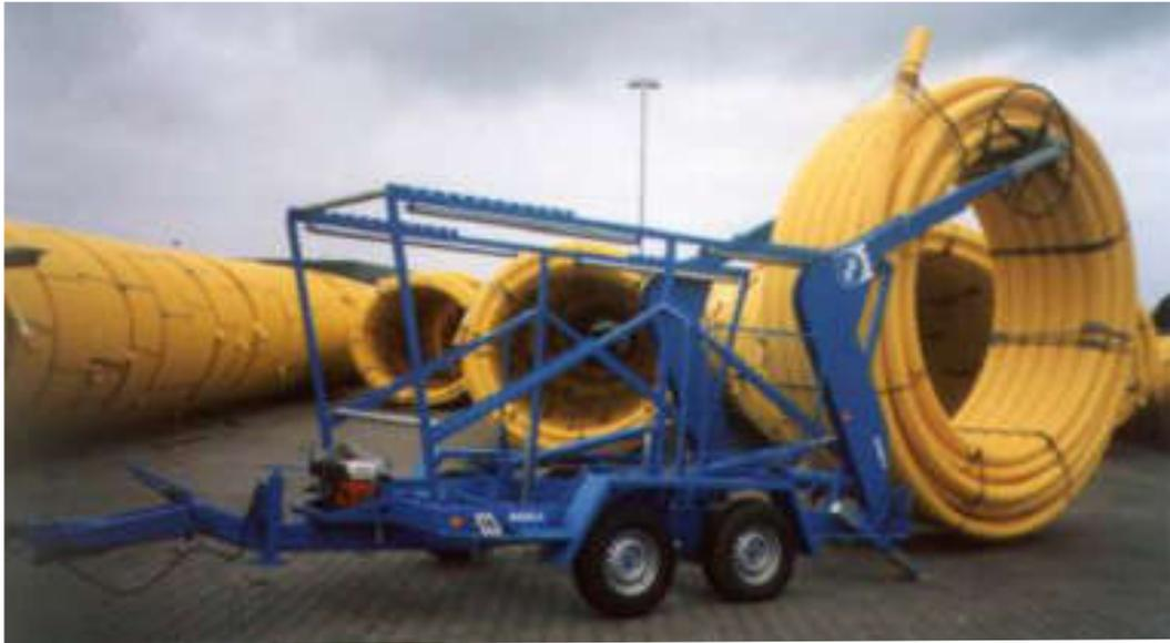
The BRT 20 is able to pick up, load and uncoil pipe coils without any help. Even laying coils can be picked up without any auxiliary equipment. Tube coils of varying diameters may be picked up with the aid of the vertical hydraulic jacks and put down on the bearing rollers. Then three guiding rollers are inserted on the inside of the coil, and the coil is ready for unreeling.
