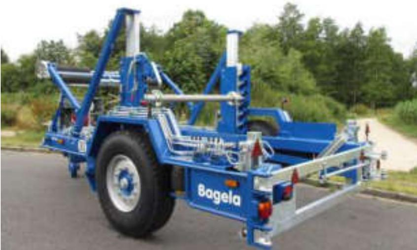
Two vertical pocket jacks, which may independently be moved up and down by an engine-driven hydraulic drive system and which are secured for transport by locking pins, lift the reel.
